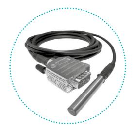
The OFT-005 measuring transducer measures relative humidity and temperature of room air. This transducer has two analogue outputs with 0...5 V. The integrated 32-bit processor and a sophisticated software allow precision at the highest operational level. Due to its modular architecture the sensors are suitable especially for industrial area
