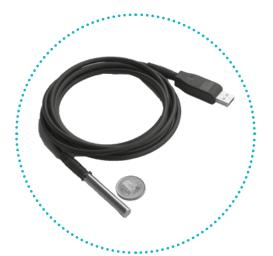
The new OHT20T USB Sensors measure relative humidity, temperature, melting point and absolute humidity. They are run directly by a USB Port of a computer. The OHT-20 is offered in three variations: Type A, B or C. Type A has a precision of +-1,5%RH for humidity and in temperature a precision up to +-0,1 degrees Celsius.
