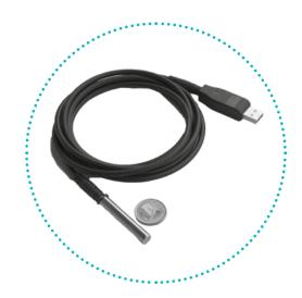
The new OHT20 USB Sensors measure relative humidity, temperature, melting point and absolute humidity. They are run directly by a USB Port of a computer. The OHT-20 is offered in three variations: Type A, B or C. Type A has a precision of +- 1,5%RH for humidity and in temperature a precision up to +-0,1 degrees Celsius.
